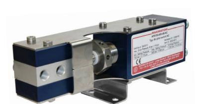
The Air Pilot Switches are designed to switch a pneumatic signal and are used to shutt-on or shut-off MAXIMATOR pumps and boosters upon achieving a desired outlet pressure. The Air Pilot Switches are available in various pressure ranges for outlet pressures from 10 to 1,000 bar. The switch does contains both functions "Air to open" and "Air to close".
