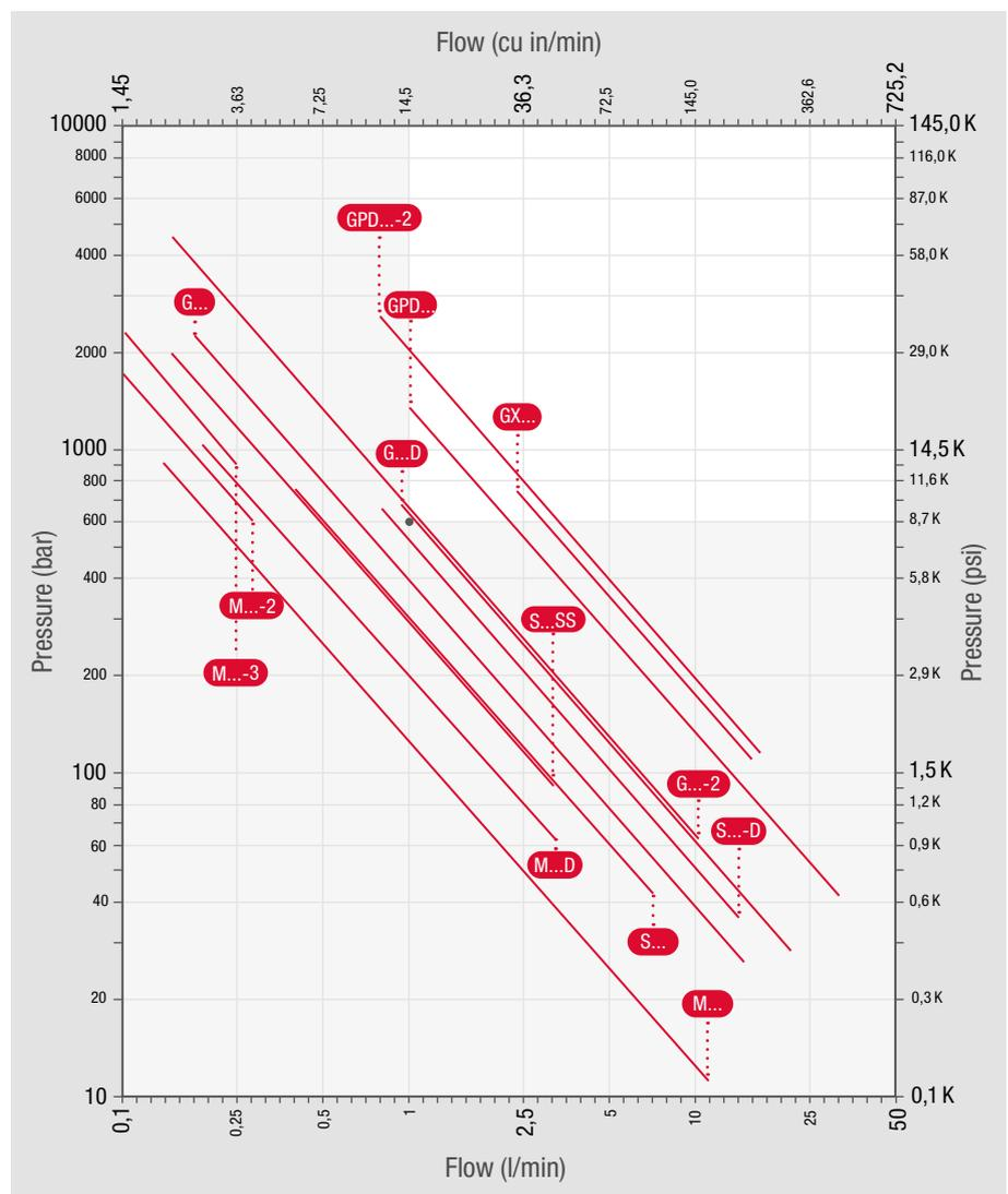
The performance data indicated here were determined with optimal flow cross-sections and the required volume flow for driving air.
