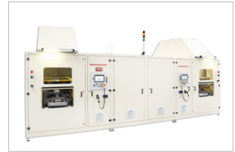
End-of-Line pressure test stand
