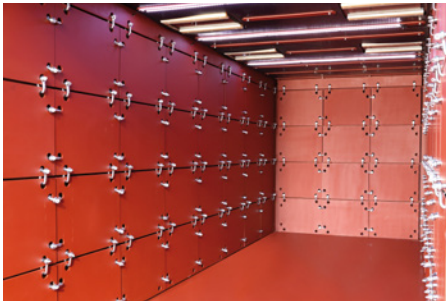
Burst test chamber with sacrificial elements
