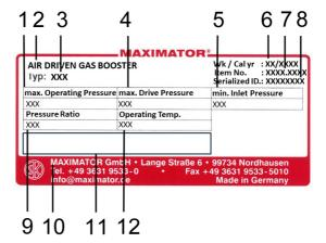
Fig. 1-1 Gas booster rating plate
