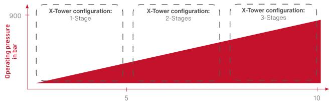
Mass Flow H2 @ 40 bar hydrogen supply in kg/h
