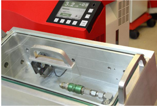
Helium leak test system during testing of a quick coupling
