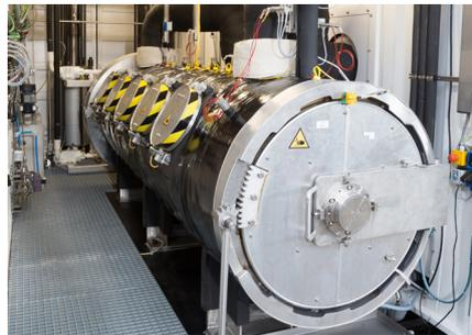
Extreme temperature pressure cycle test stand
