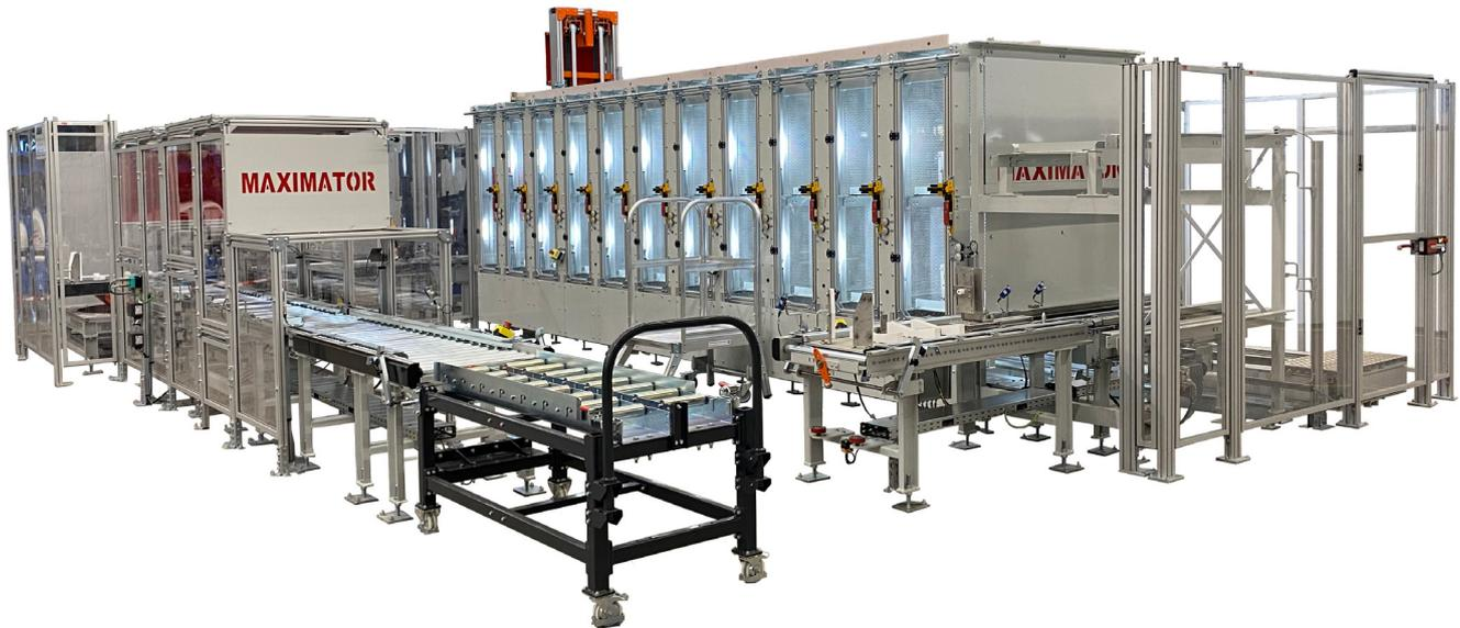
Fully automated leak test stand
