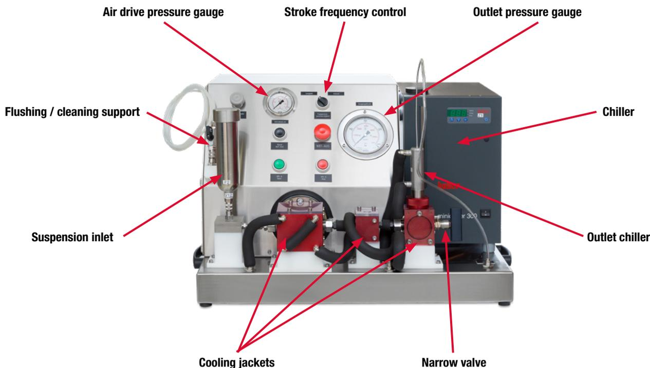
The Maximator high pressure homogenizer HPL6 is designed for energy-efficient, continuous production of superfine emulsions. The HPL6 system achieves the homogenizing effect by means of fully adjustable decompression of the liquid from max. 4,200 bar to an ambient pressure.
