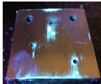
Fluorescing particulates and hydrocarbon residues on a not yet cleaned part become visible under ultraviolet light.
