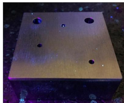
A specially cleaned part for oxygen applications under ultraviolet light.
